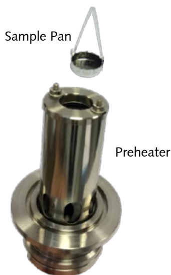
High temperature pre-heater for in-situ degassing/regeneration of samples up to 400°C. Temperature is measured by Pt-100 thermocouple, which is placed below the stainless steel sample pan.
