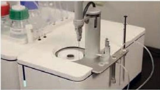
If the cell is loaded, move the pipette into the cell.
