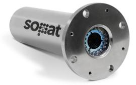
The InView system is equipped with a color camera and is suitable for many different particle detection tasks. The InView is equipped with a ring of LEDs, but additional LED panels can be used to illuminate the objects in different angles and distance. To reduce fouling on the InView window, we optionally provide a purging device which is mounted on the flange provided.
