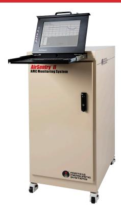
The AirSentry® II Multi-point Monitoring System is the most advanced airborne molecular contamination (AMC) monitor available, utilizing sensitive and responsive ion mobility spectrometry to detect and characterize airborne molecular contamination from multiple locations within a cleanroom. The system features a 16- or 30-point manifold sampling system and an on-board industrial computer with secure software and communications.
