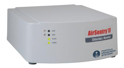
The AirSentry II family of ion mobility spectrometers detect and alert users to small concentrations or changes in airborne levels of chlorides, acids, amines and ammoniacontaining species. With parts-per-trillion (ppt) sensitivity, these point-of-use sensors provide fast response, increased detection selectivity and repeatable performance.
