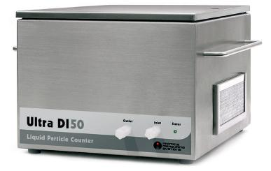
The Ultra DI® 50 Liquid Particle Counter is designed specifically for de-ionized (DI) water systems and will count and size contaminants as small as 20  $\mu m$ . Larger sample volumes and ultra-low zero counts detect smaller excursions with more relevant statistical data, while shorter sample intervals speed up your analysis time.
