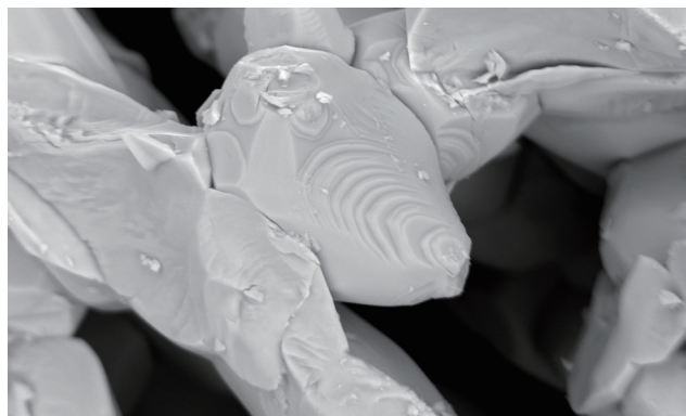
Strontium barium titanate ceramics Acceleration voltage: 10 kV/magnification: ×10000
